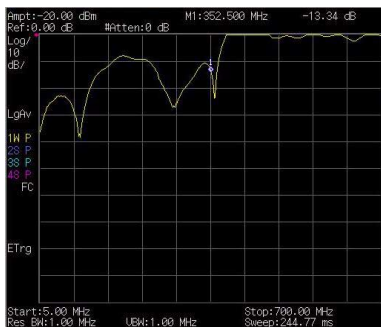
Figure 3-22 Measuring the Return Loss of the Filter
